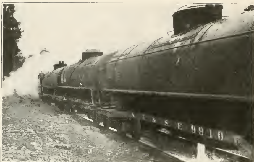
Water tank cars for hauling water ninety-eight miles from Flagstaff, Arizona, to the Grand Canyon National Park. No water is available on the top rim of the Canyon.
